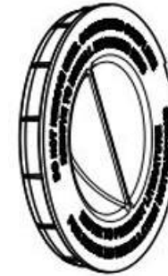
PROTECTIVE CAP CONCRETE NICHE CAP
