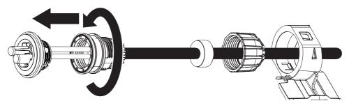
LEAVE THESE PARTS DISASSEMBLED UNTIL AFTER ADDING LANOLIN
