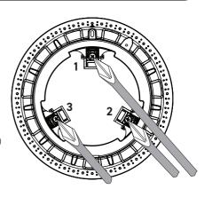
AS THE CAM LOCK SCREWS TIGHTEN, THE CAM LOCKS WILL MOVE IN AND UP, PULLING THE NICHE ADAPTOR FIRMLY INTO THE NICHE THE ADJUSTMENT RANGE OF THE CAMS ACHIEVE P.C.D. 7 ½" - 8 ½" (190-210mm) (APPROX.)
