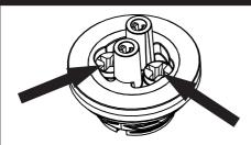
USE A MANUAL PHILLIPS HEAD SCREWDRIVER TO ENSURE THAT THE 2 SCREWS INDICATED ARE FULLY SEATED. PROCEED TO STEP 8.
