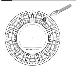
USE A SCREWDRIVER TO LOOSEN THE SCREW
