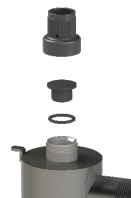
Pressure Test Cap Installation
