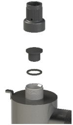
Figure 3. Pressure Test Cap Installation
