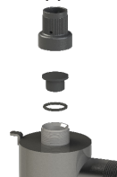
Pressure Test Cap Installation
